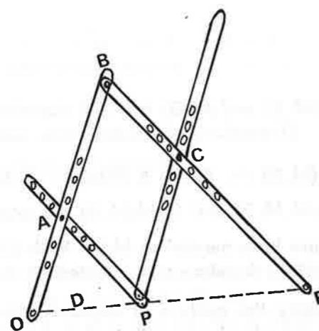
A pantograph can be made from strips of stout card and paper fasteners, or from **Meccano**, or from strips of peg-board (Fig. 10.27).
